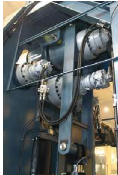
2-4 Drive Rodillo superior Ø 140mm - 430mm
